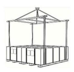
Use reasonable hoisting jigs, hoisting allows up to 2 supporting modules at a time. Before hoisting, confirm whether the pallets and cartons are damaged and whether the hoisting ropes are strong and firm. When the hoisting is about to touch the ground, two of them will straighten the carton and gently place it on a relatively flat position
