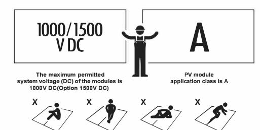
\* When Module exposed to sunshine or other lights, it can produce DC, in this case it may cause electric shock hazard if touch electrical parts
