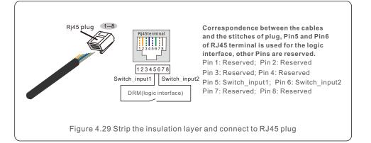
3.Connect RJ45 to DRM (logic interface).
