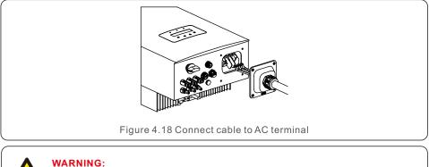
When assembling the AC terminal, be careful not to cut the insulation layer of the wire, or it might lead to poor contact.
