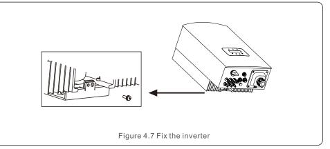
The are two holes at the bottom of bracket, one to fix the inverter, another for the lock. **The diameter of the lock should be less than 0.27in (7mm).**
