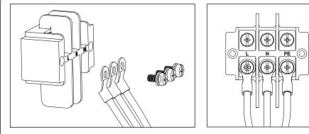
Figure 4.16 Copper-aluminum transition terminal
