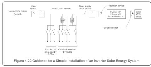
The RCD should be in parallel connection between the consumers mains and the solar supply.
