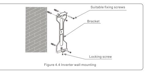
2.Make sure the bracket is horizontal and the mounting holes (in Figure 4.4 and Figure 4.5)
